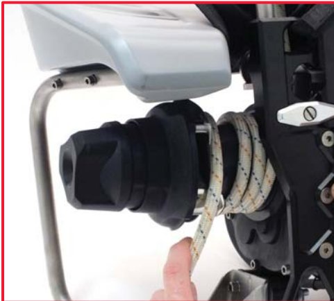
8. Pass the rope over the stripper arm.
