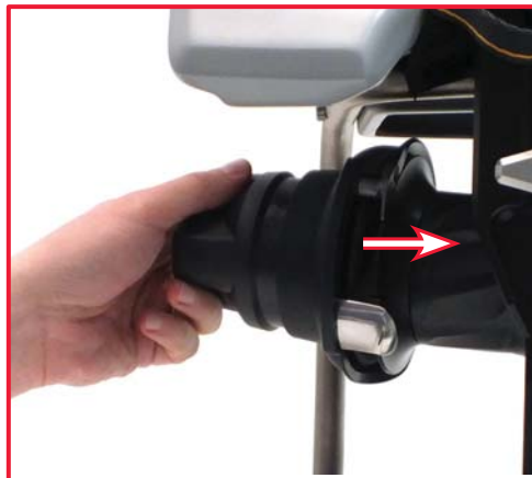
Check that the rope grab knob is working by rotating it and releasing it (CLOSE JAW).
