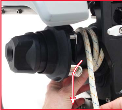
7. Wind the rope clockwise around the winch drum.
