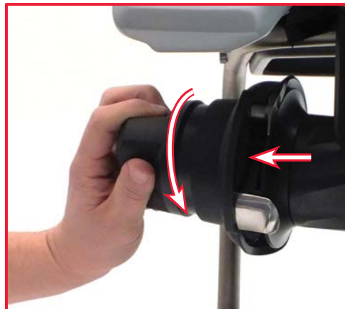
Check that the rope grab knob is working by rotating it and releasing it (OPEN JAW).
